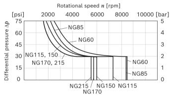
Minimum pressure – pump operating mode (inlet)
