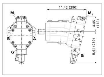
38 **A6VM series 71** (Americas) | Axial piston variable motor Dimensions, size 85
