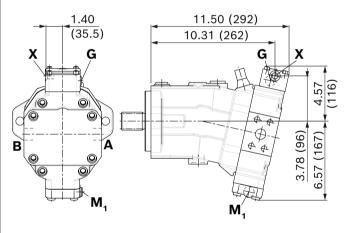
▼ HZ7 – Two-point hydraulic control, negative control
