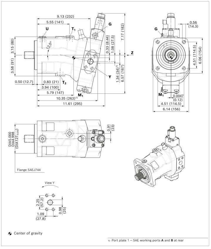
34 **A6VM series 71** (Americas) | Axial piston variable motor Dimensions, size 85
