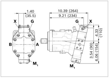
30 **A6VM series 71** (Americas) | Axial piston variable motor Dimensions, size 60
