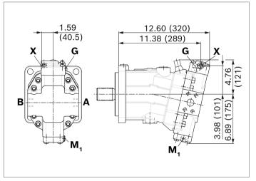
▼ HZ7 - Two-point hydraulic control, negative control
