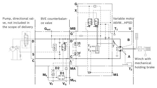
68 **A6VM series 71** (Americas) | Axial piston variable motor BVD and BVE counterbalance valve
