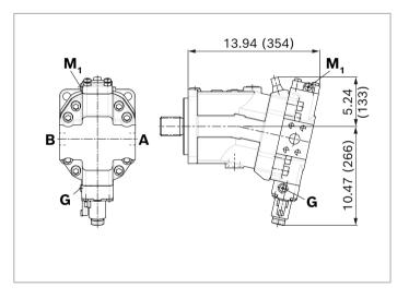
56 **A6VM series 71** (Americas) | Axial piston variable motor Dimensions, size 170
