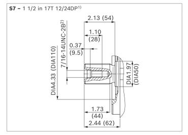
1) Involute spline according to ANSI B92.1a, 30° pressure angle, flat root, side fit, tolerance class 5
