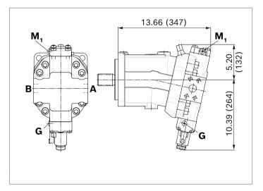
50 **A6VM series 71** (Americas) | Axial piston variable motor Dimensions, size 150
