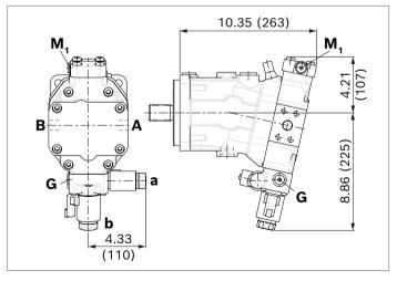
1) Port plate 1 - SAE working ports **A** and **B** at rear
