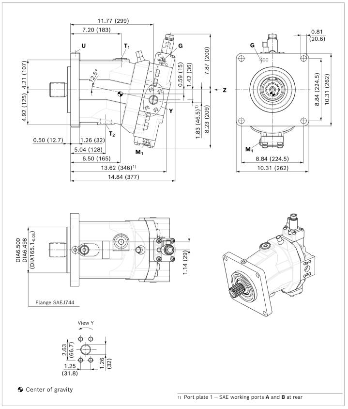
58 **A6VM series 71** (Americas) | Axial piston variable motor Dimensions, size 215
