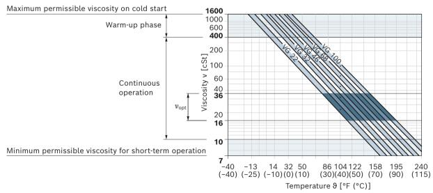
This corresponds, for example on the VG 46, to a temperature range of +39.2 °F ... +185 °F (+4 C ... +85 °C) (see selection diagram) 3) If the temperature at extreme operating parameters cannot be adhered to, please contact us.
