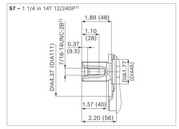
Involute spline according to ANSI B92.1a, 30° pressure angle, flat root, side fit, tolerance class 5
