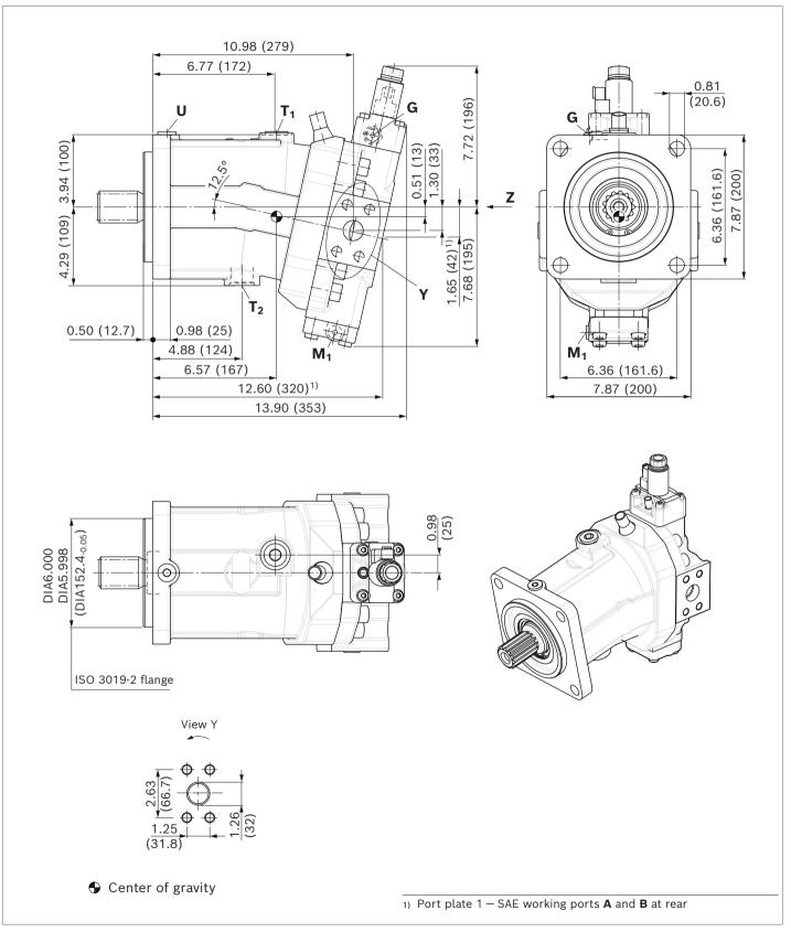
46 **A6VM series 71** (Americas) | Axial piston variable motor Dimensions, size 150
