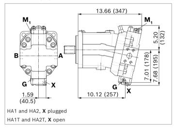
▼ HA1R1, HA2R2 – Automatic high-pressure related control, positive control, with electric override and electric travel direction valve
