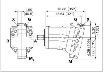
▼ HZ5 - Two-point hydraulic control, negative control
