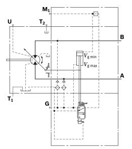
▼ Circuit diagram EP5, EP6 (negative control)
