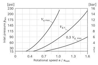
This diagram is valid only for the optimum viscosity range from  $v_{opt}$  = 36 to 16 cSt.
