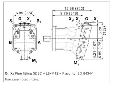
▼ **DA1, DA2** – Automatic speed related control, negative control, with electric travel direction valve and electric V<sub>g max</sub> override
