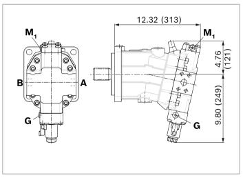
1) Port plate 1 - SAE working ports  ${\boldsymbol A}$  and  ${\boldsymbol B}$  at rear
