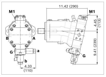
1) Port plate 1 - SAE working ports  ${\bm A}$  and  ${\bm B}$  at rear
