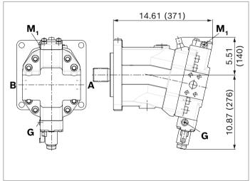
62 **A6VM series 71** (Americas) | Axial piston variable motor Dimensions, size 215
