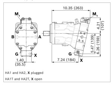
▼ HA1R1, HA2R2 – Automatic high-pressure related control, positive control, with electric override and electric travel direction valve
