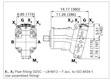
▼ DA1, DA2 – Automatic speed related control, negative control, with electric travel direction valve and electric V<sub>g max</sub> override
