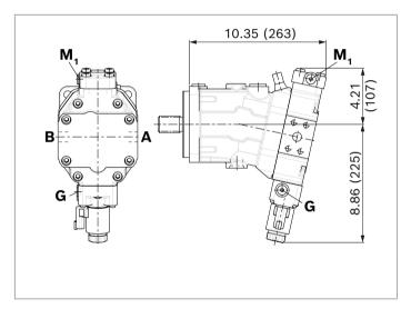
▼ **DAO** – Automatic speed related control, negative control, with hydraulic travel direction valve
