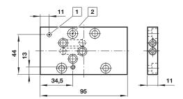
1 Two screws M4 x 50 mm deep to mount the VP50 onto the manifold 2 Four screws M6x16 mm deep to mount the manifold onto the iso subbase
