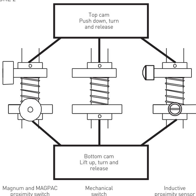
**Switch adjustment (four switches, no CS transmitter option)**
