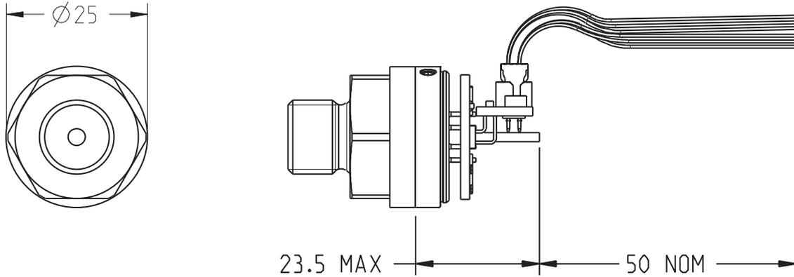
GAUGE SENSOR WITH PB PRESSURE CONNECTOR SHOWN
