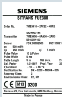
FUE380 transmitter label (with MID first verification)
