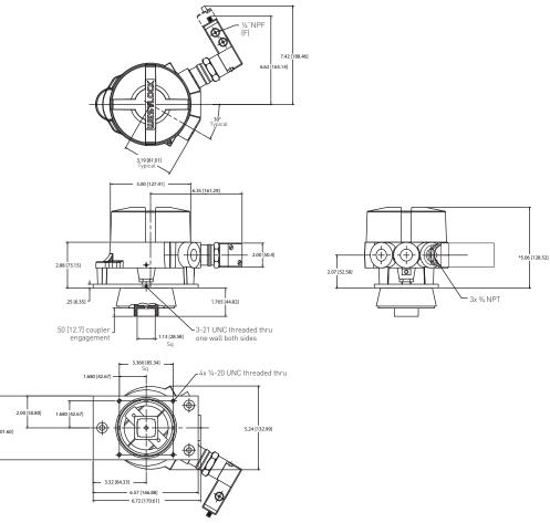
Dimensions in inches, metric dimension (mm) in parentheses Solenoid valve dimensions are indicative only and are dependent on solenoid valve selected
