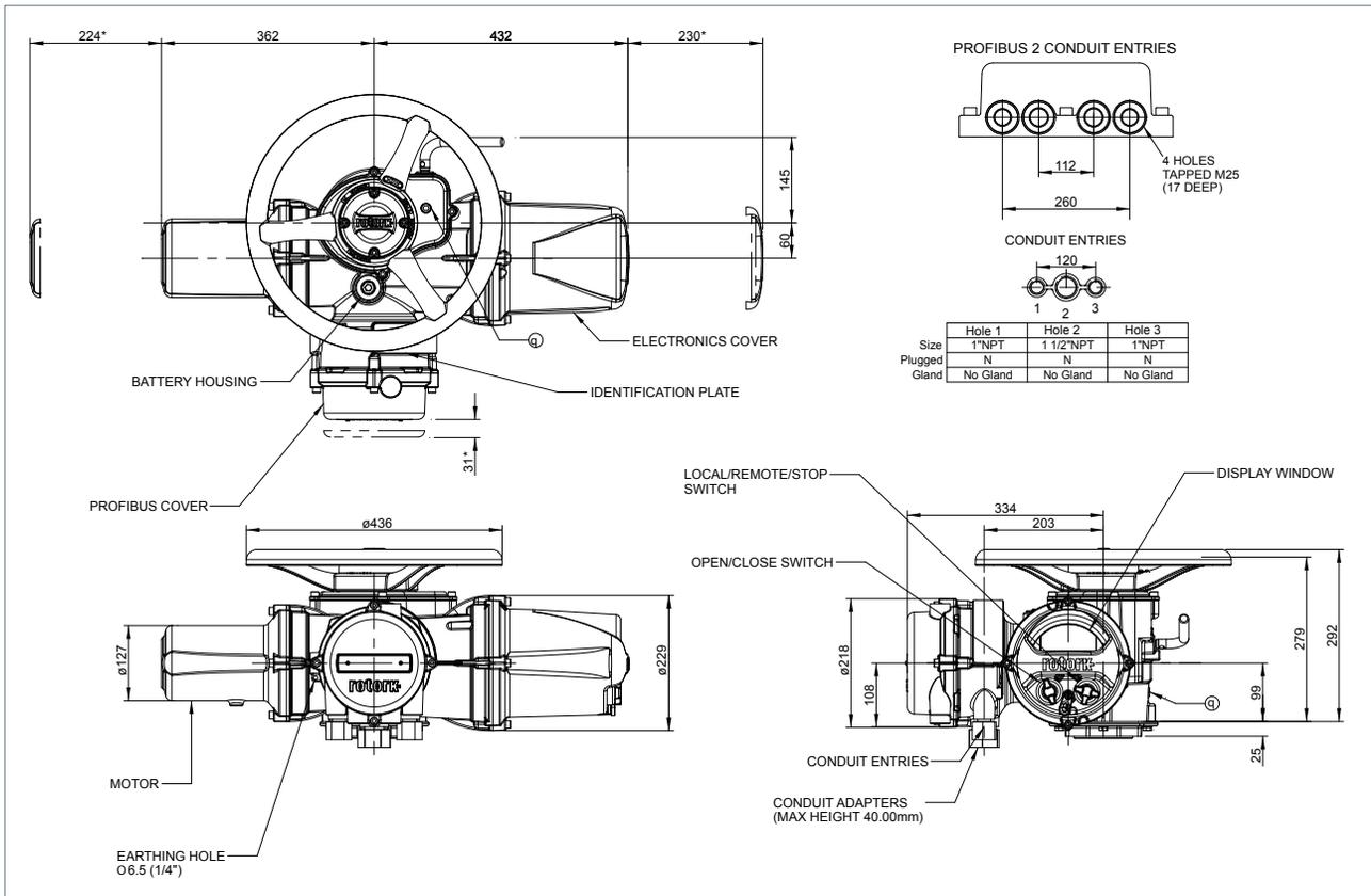
*IQ3 with optional highway termination module fitted*
