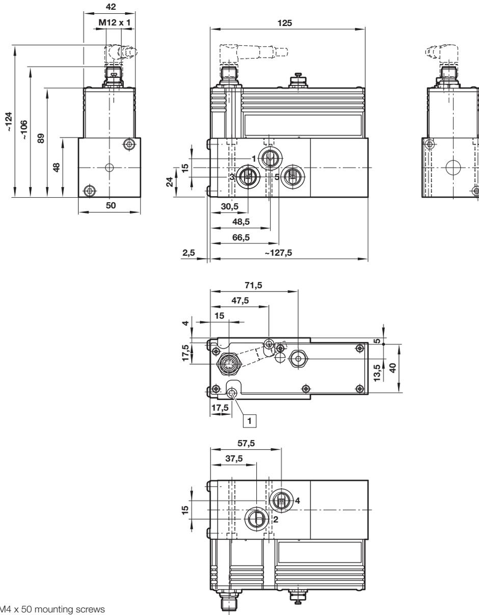
1 Valves are delivered with M4 x 50 mounting screws
