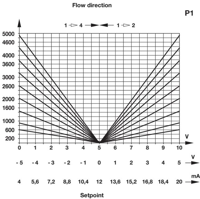
Flow-rate as a function of setpoint value at constant pressure P1=6 bar, P2, P4 = 5 bar:
