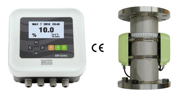
The Clamp-on density measurement guarantees fit-and-forget and reliable measurement with almost no influence on measuring medium. Different from other density meters, this technology doesn't affected by pressure, corrosion, nor abrasion. As the clamp-on sensor can be mounted outside of pipe line even under flow-running condition, the user neither need to stop their process nor to consider additional by-pass line.
