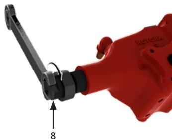
6. Verify the newly obtained angular position with one closing stroke.
