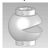
Specially engineered reduced Cv trims can control very low flows with high accuracy. The trim orifice is continually increasing which also acts as a self flushing feature.
