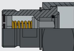
Connection for analytic instruments, model GCG-20
