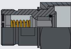
**Connection for analytic instruments, model GCG-20**
