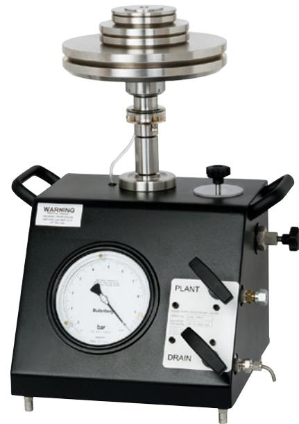
Hydraulic pipeline tester, model 80
