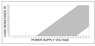
The diagram shows the optimum ratio between load and power supply for transmitters with 4...20mA output.
