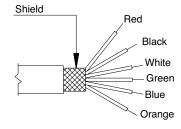
Shielded cable 6x0,25 - 1m Protection IP65
