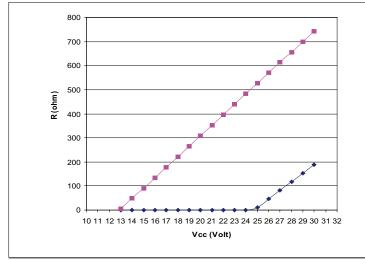
The diagram shows the optimum ratio between load and power supply for transmitters with 4...20mA output.
