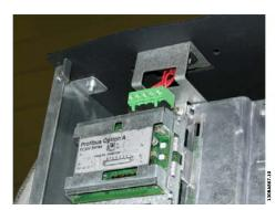
Figure 3.53: Top connection for serial communication bus.
